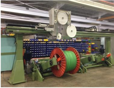
MGS / HALL designs and manufactures product handling solutions which include Payoffs, Takeups, Dancers, Accumulators, Measuring Machines, and Capstans to handle most any product from sensitive optical fiber to 1000MCM (507-mm²) power cable. We also can handle odd shapes, tubing, ribbon, and tape.
