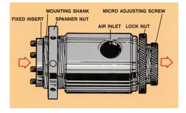
The Multiple Wipe is equipped with mated pairs of interchangeable inserts, from 1/8 inch to  $1\frac{1}{2}$  inch ID. These are divided into two ranges; the smaller one covering from 1/8 inch to  $\frac{1}{2}$  inch ID, and the larger one covers from  $\frac{1}{2}$  inch to  $\frac{1}{2}$  inch ID.
