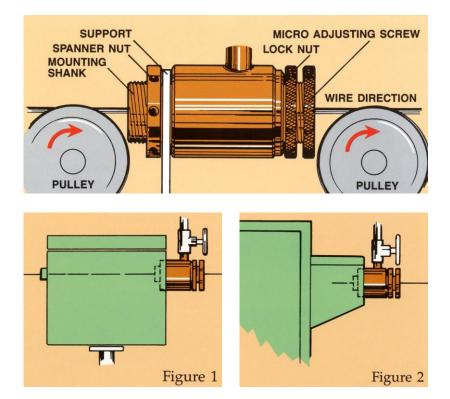
For additional noise reduction, the Air Wipe can be mounted on a metal drainage box. Air Wipes are often mounted in a drainage box attached to the side of the Capstan enclosure. They can also be mounted directly on the side of the Capstan enclosure. (See Figure 1 and Figure 2.)
